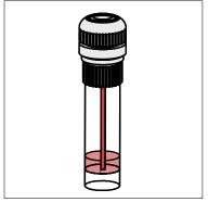
Insert the filled glass capillary into the solution Before twisting off the cap, let the sample mixture settle back to the bottom of the solution bottle. Only then twist off the cap.
