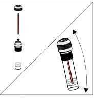
bottle and screw the cap back. Mix the content of the solution bottle by turning it gently upside down several times until the blood from the glass capillary tube is mixed with the solution
